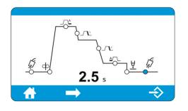
**Miller 4TS trigger functionality** – Gives access to hot start or cold start from the torch trigger
